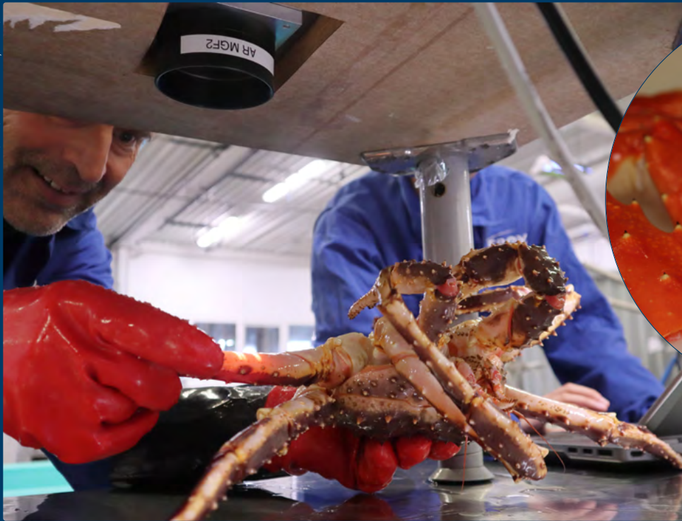
(Photo to the left) Meat content in cooked crab leg to match with the NIR measurement. (Photo above) Measurement of meat content in live king crabs with NIR spectroscopy.
