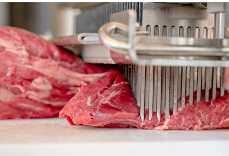
This is how mechanical tenderisation takes place in Nofima’s Meat Pilot Plant. Small knives that are placed closely together cut small incisions in the meat.
