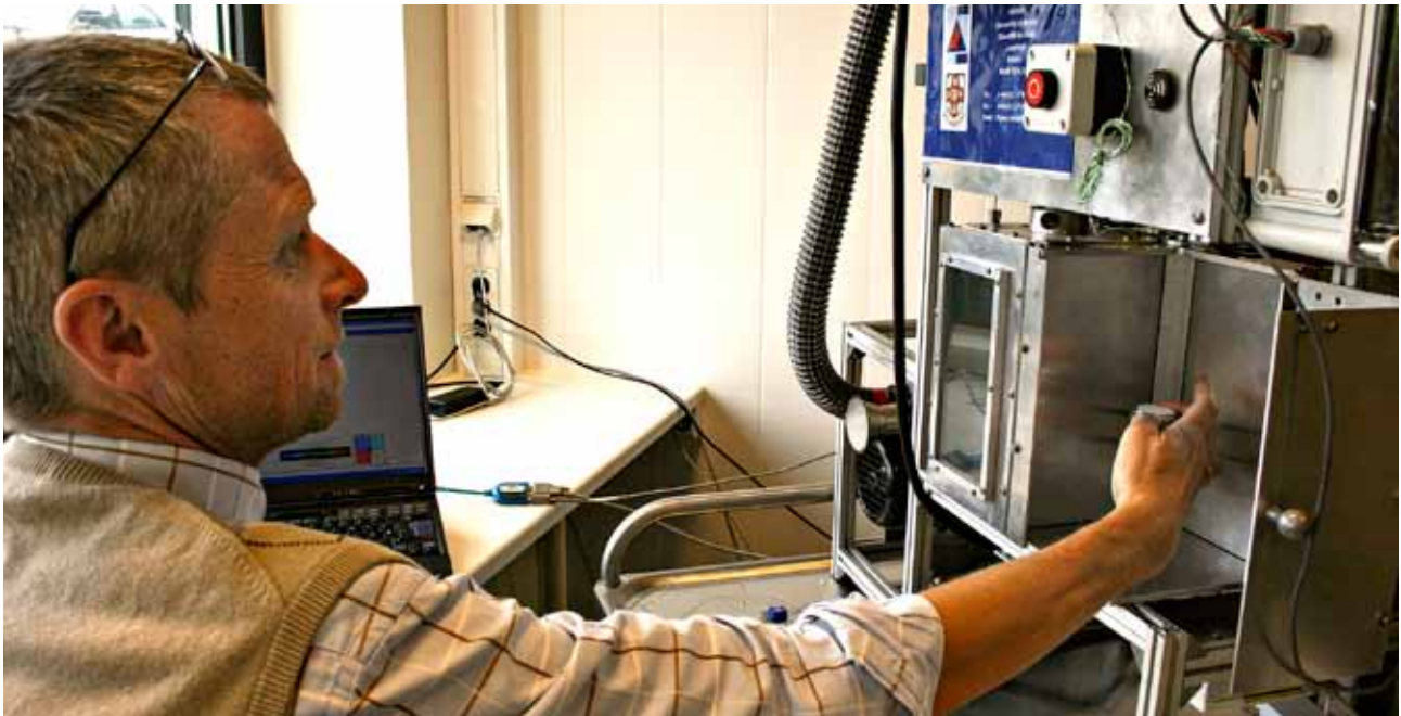
Torstein Skåra places a sample in the steam chamber of the test rig. It is closed and steam is injected from above at given time intervals.
