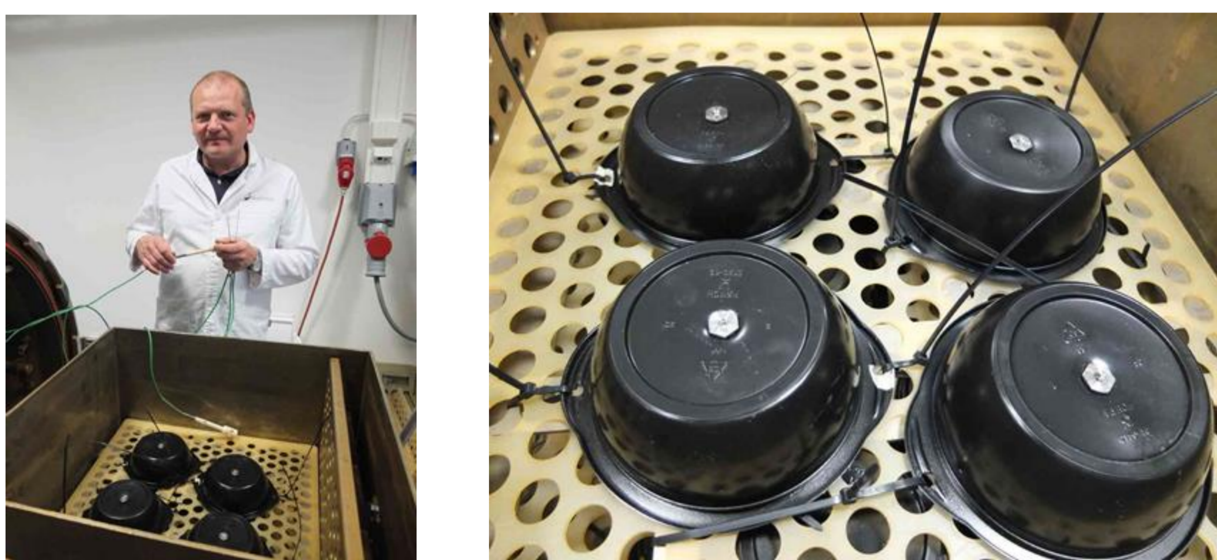
Figure 1 Temperature logging in industrial produced stew in the autoclave
