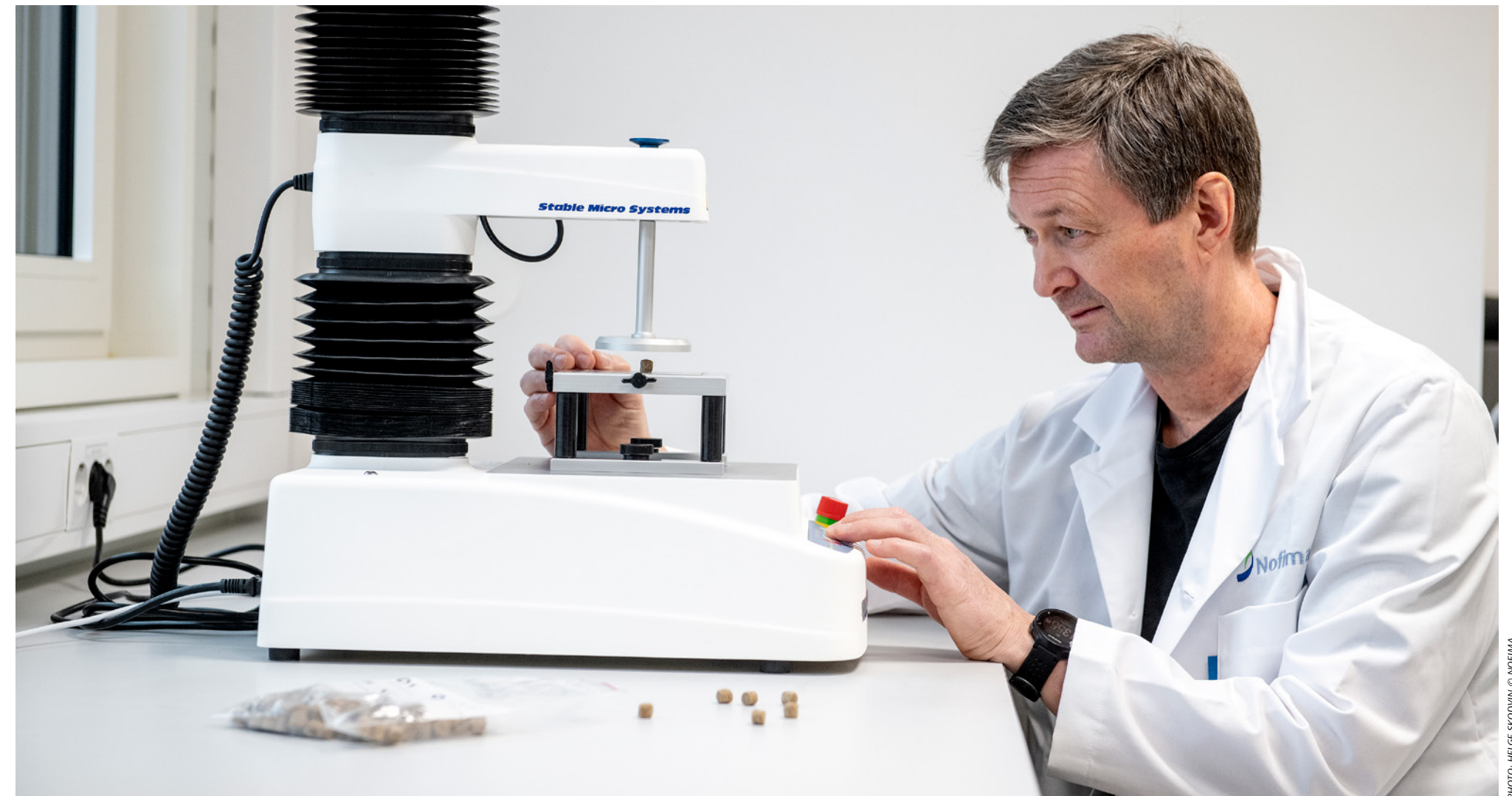
Tor Andreas Samuelsen measure the feed pellets’ fracture strength (hardness).
